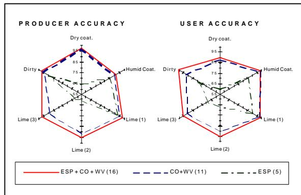
Figure 7. producer and user accuracies for the classification of 6 types of materials using three different sets of features: spectral (ESP), texture cooccurrence and wavelets features (CO+WV), and all combined (ESP+CO+WV).
