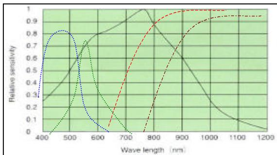
Figure 1. Spectral sensitivity response of the CCD (continuous) and transmission curves of the 4 spectral filters (dashed).
