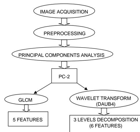
Figure 4. Process of texture feature extraction ( $PC-2$ : 2<sup>nd</sup> principal component;  $GLCM$ : grey levels cooccurrence matrix;  $DAUB4$ : Daubechies-4).
