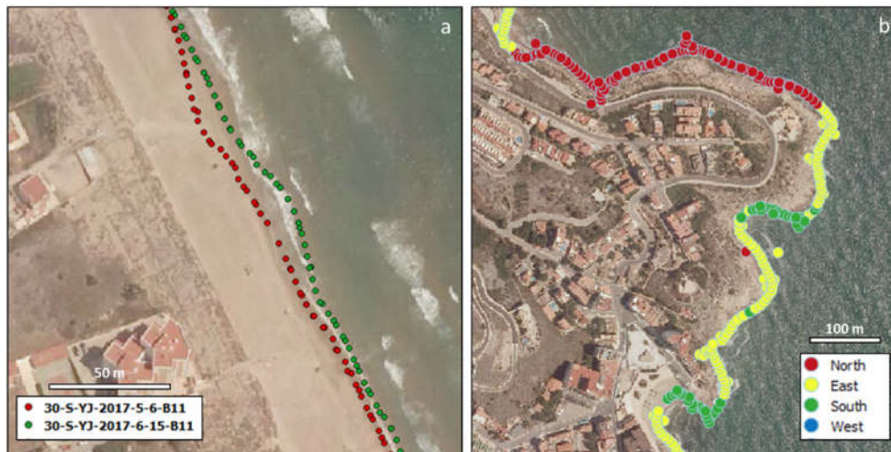
Figure 10. Extracted shorelines (10a) and main beach orientations (10b).
