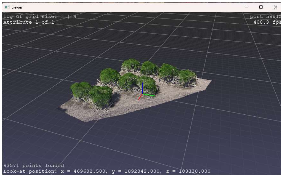
Figure 4. Class3Dp software visualising a point cloud of 41.7 million points.
